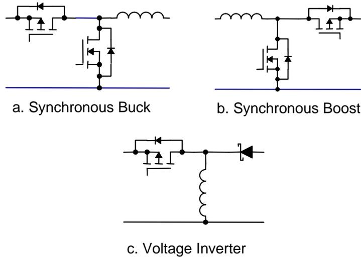
Figure 1. DC-DC topologies using P- channel MOSFETs
