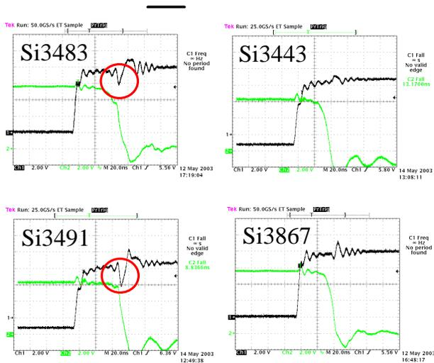
Figure 6. Turn off waveforms, Gate (black), Drain (green)
