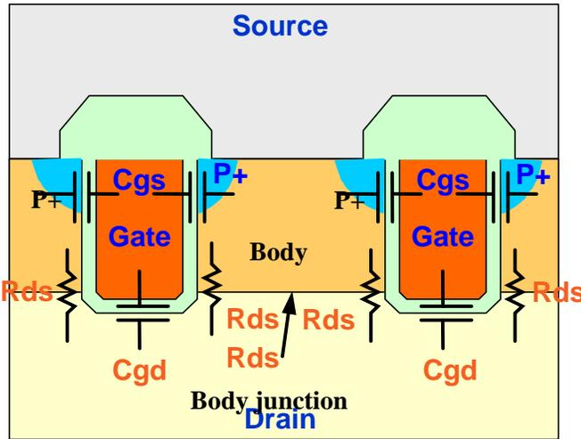
Figure 4. Cross section of Trench MOSFET
