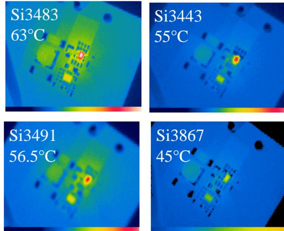
Figure 7. Thermal images at 2-A output
