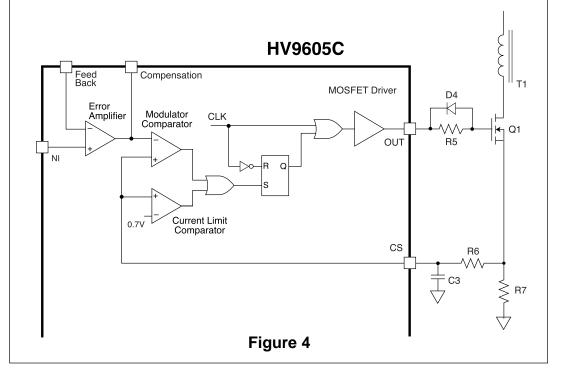
the modulator comparator, the supply could become unstable. Secondly, the turn-on spike, due to turning on the MOSFET, could also falsely trip either of the modulator or current limit comparator. This too, would result in unstable power supply operation.
